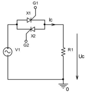
**Datos:**  $R_1 = 220 \Omega$ ;  $U_{red} = 220 \text{ V}$ ;  $f = 50 \text{ Hz}$
